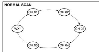
\* Previously selected weather channel when weather alert function is ON.
