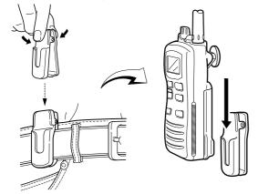
3 Once the transceiver is locked in place, it swivels.
