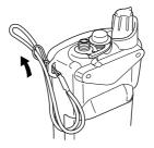
Pass the handstrap through the loop on the top corner of the transceiver as illustrated at left. Facilitates carrying.
