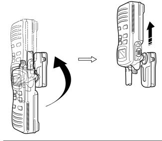
⚠ CAUTION!: HOLD THE TRANSCEIVER TIGHTLY WHEN HANGING OR DETACHING THE TRANSCEIVER FROM THE BELT CLIP.
